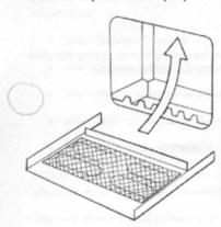
Place the left hand side brick in place, followed by the right hand. The top baffle can then be placed correctly and the rear brick inserted.
