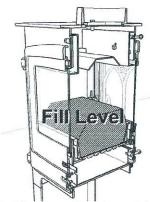
The double-sided stove has air controls on both sides. Take very great care to guard against the possibility of overheating ('overfiring') which can lead to permanent damage. Always keep the stove under close observation, especially within the first 20 minutes of lighting or refuelling.
