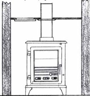
Typical Rear Flue Installation with clean out door
